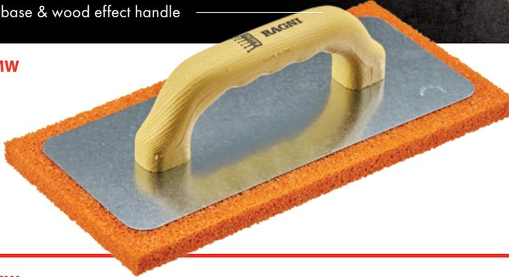
Float soft wide sponge pores deal for dampening walls. Smooths over plaster to open up surface before final trowel finishing.
